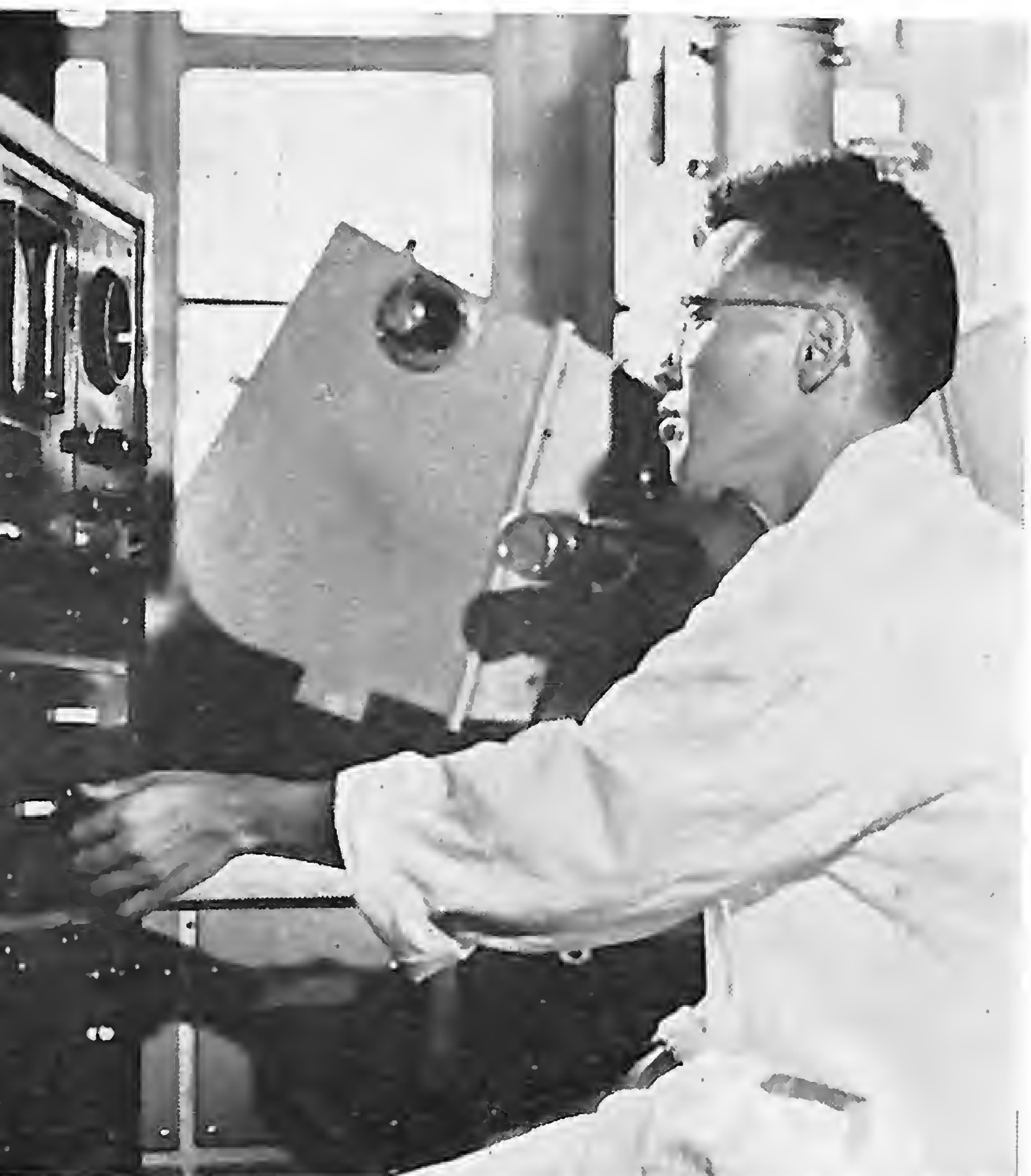
An electron probe X-ray micro-analyser made in the Nanking Chiangnan Optical Instruments Factory is tested and aligned.
